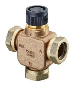
The Tri CTR is a three port valve which can be used as a diverting or a mixing valve. When used as a diverting valve the Tri CTR has one inlet (AB) and two outlets (A and B). Depending on the stem position the flow is diverted to either outlet A or outlet B.
