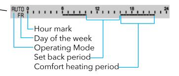
Programming is arranged in 10 minute blocks with three heating periods per day.
