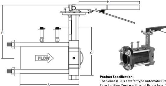
The Series 810 is a wafer type Automatic Pressure Independent Flow Limiting Device with a full flange face. The Series 810 is designed to fit between two ANSI Class 125 flanges. The Series 810 is supplied with one or more stainless steel flow limiting cartridges that can be removed for cleaning, inspection, and, if necessary, cartridge exchange. The Series 810 has two pressure/temperature ports. The Series 810 has a butterfly valve for positive shutoff.
